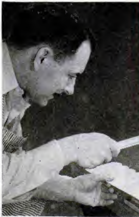
Hand-operated punch makes clean, round holes for rivets or decorative effects. Square dies are available for certain type punches, also accessory shear blades in various sizes
